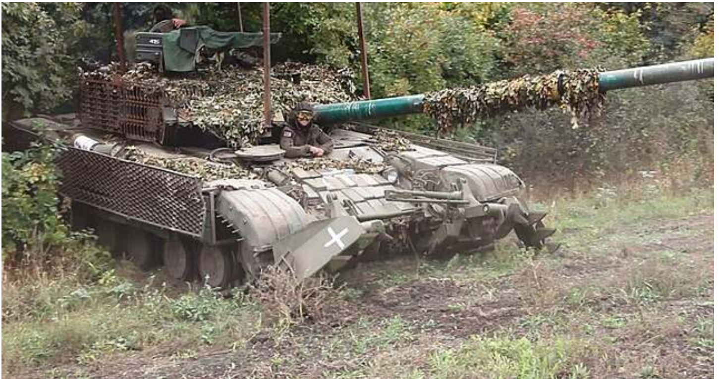
Figure 1: Despite the proliferation of drones, tanks like this Ukrainian T-64 have opted for improvised protective cages rather than disappear from frontline combat altogether. АрміяInform, CC 4.0
